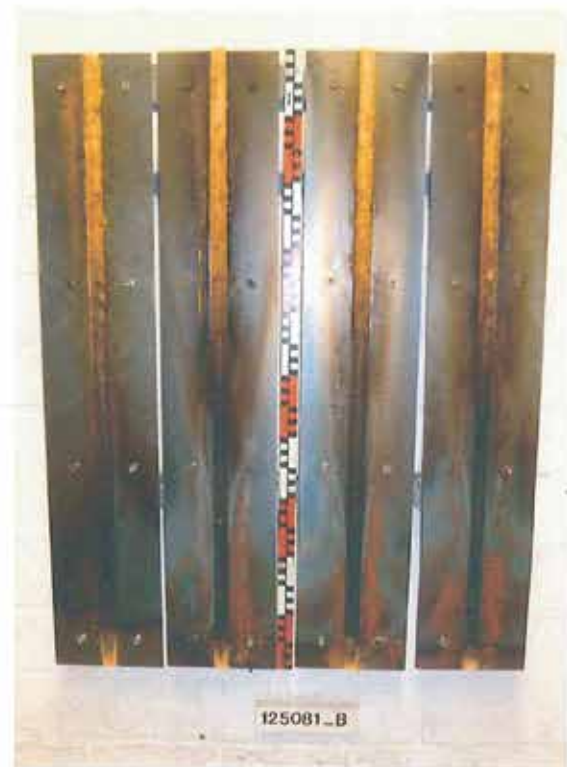
Figure 4: Appearance of specimen B after 10-minutes burning
