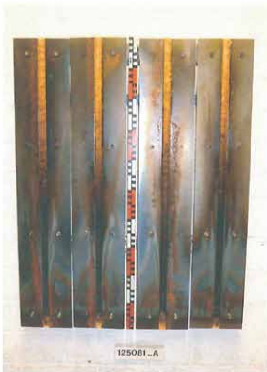
Figure 3: Appearance of specimen A after 10-minutes burning
