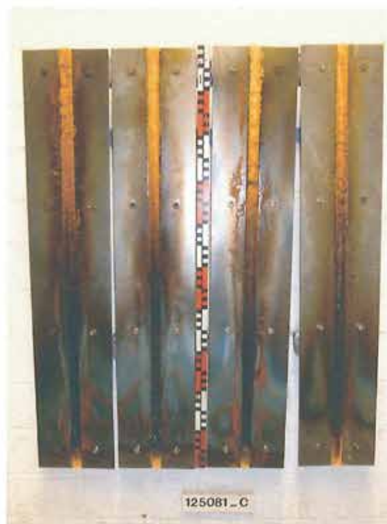
Figure 5: Appearance of specimen C after 10-minutes burning
